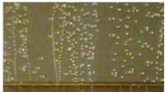
(f) wrapped smooth tube ( \theta = 2^\circ ), q=900 \text{ W/m}^2 , R-134a
