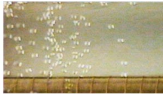
(b) wrapped smooth tube ( \theta = 2^\circ ), q=900 \text{ W/m}^2 , R-600a
